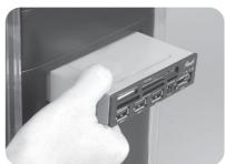
B-2. Insert the Internal card reader into the drive bay until it is in line with front panel of the chassis.
